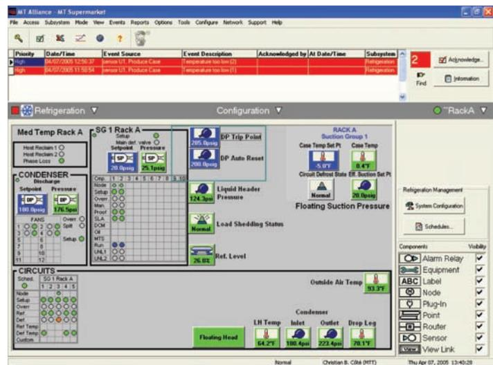
Display and modify compressor, condenser, suction group and refrigeration circuit status and values from a single screen
